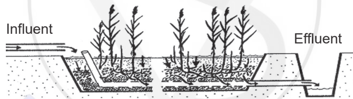
Figure B: Horizontal flow
